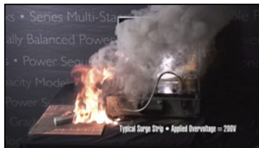
Standard power strips are not equipped to handle sustained overvoltage conditions.
