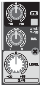
Fig. 2.6: The FX send/balance/level controls
